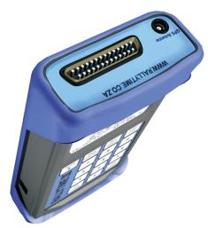
All clocks get a master time signal from the GPS satellites before a control, then use an internal quartz timebase for up to 8 hours.
